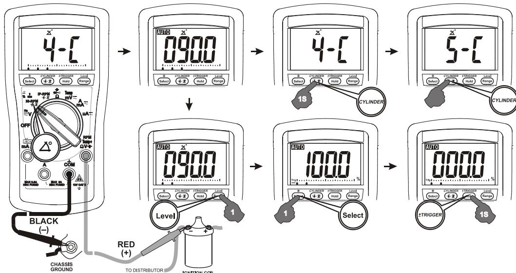
Number of cylinders defaults at 4 cylinders. Press Cylinder button for one second or more to display the cylinder setting, and press momentarily again within one second to select the number of cylinders from 1 through 12 to match the engine under test. Adjust the dwell angle according to the procedures outlined in your vehicle service manual. Re-check the timing whenever the dwell angle has been adjusted.
