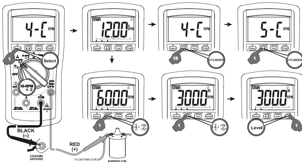
Press  $\overset{\text{4}}{1}$   $\overset{\text{2}}{2}$  button momentarily to select through **RPM**  $\overset{\text{4}}{1}$  for 4-stroke, **RPM**  $\overset{\text{2}}{2}$  for 2-stroke and DIS, and **RPM**  $\overset{\text{2}}{2}\text{M}$  for special 2-stroke waste ignition engine
