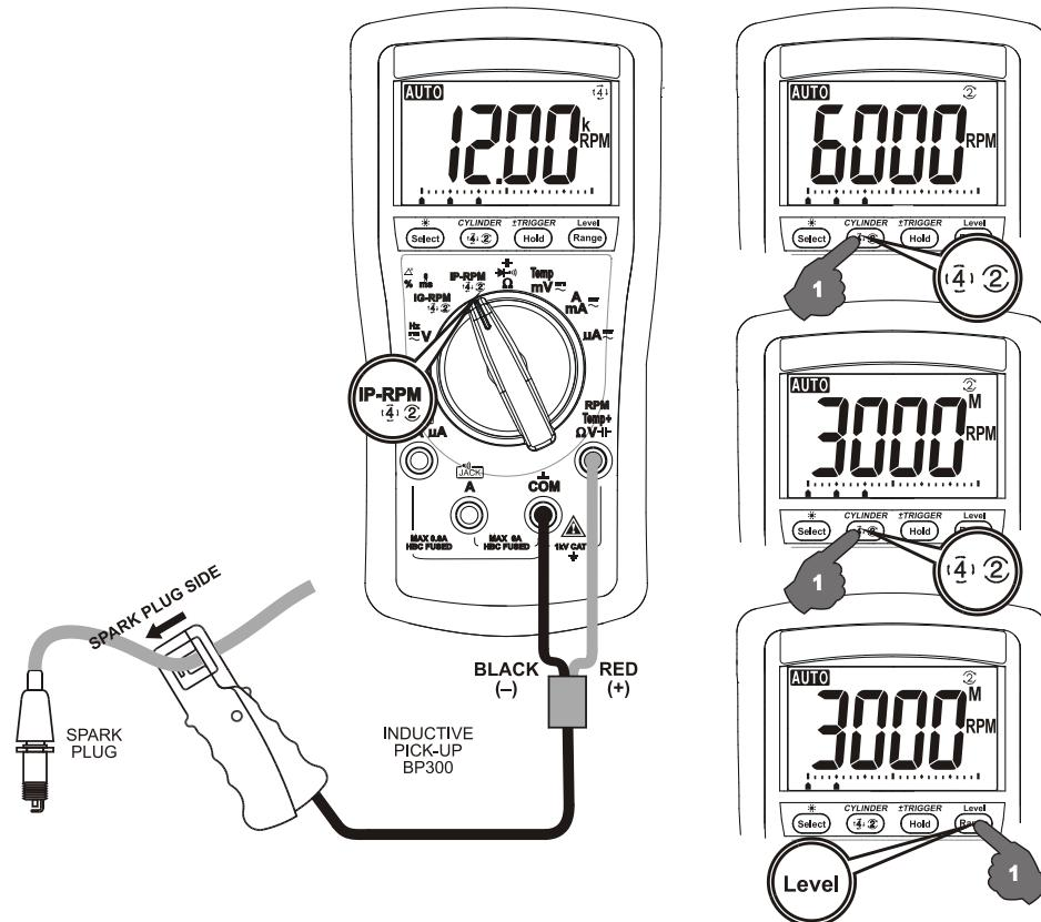
Press  **$(1)$   $(2)$**  button momentarily to select through **RPM<sup>(1)</sup>** for 4-stroke, **RPM<sup>(2)</sup>** for 2-stroke and DIS, and **RPM<sup>(2)</sup> M** for special 2-stroke waste ignition engine
